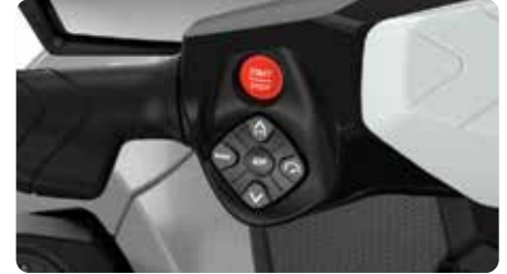
iDF – Intelligent Debris-Free Pump System (optional) An innovative, industry-first system that allows you to free your pump of weeds and debris with intuitive handlebar-activated controls.
